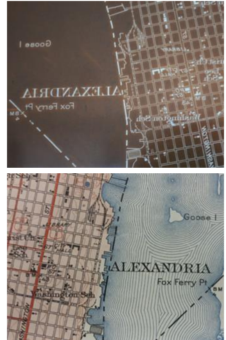
Figure 1. A portion of an engraving (top) used to print the black ink for a USGS topographic map (bottom). (Photo courtesy of Bruce Geyman.)
