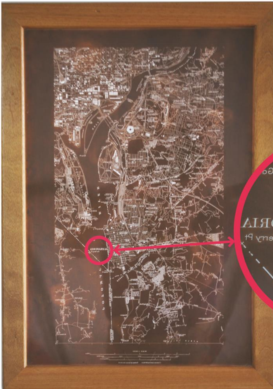
Figure 2. (Above) Typical display on a wall of three cleaned, polished, enhanced, and framed engravings. These engravings are some of those used to print the USGS 1:31,680-scale topographic map "Washington, D.C. and vicinity". From left to right are the engravings used to print cultural, transportation, and boundary features and text with black ink; contours with brown ink; and hydrography with blue ink. (Photo courtesy of Bruce Geyman.)
